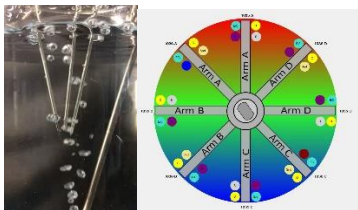
Figure 1: Local Array Probes and Cross-section of 2 combined Array Production Logging Tools.
