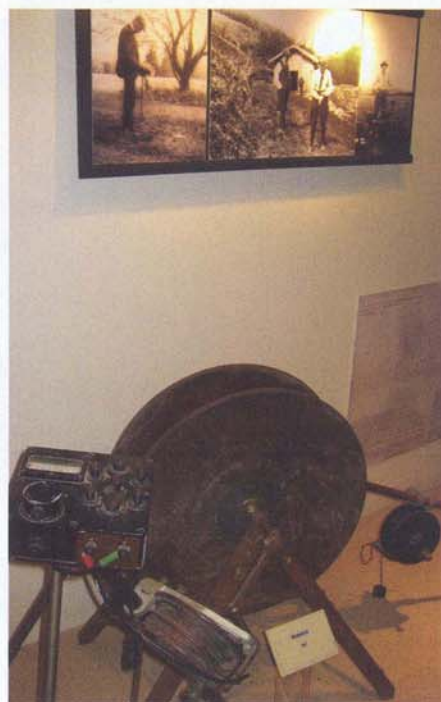
This early logging kit in the Schlumberger museum showed a simple setup with the black box that measured resistivity and reels that handled the cables. (Photos by Don Lyle)
